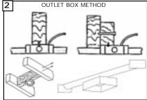
WARNING – Risk of fire, electric shock, or personal injury, The fan in this box may be either directly supported from a structural framing member of a building and/or may be mounted to an outlet box marked acceptable for fan support of 31.8 kg. (70 lbs.) or less. Most outlet boxes commonly used for the support of luminaires may not be acceptable for fan support and may need to be replaced. Consult a qualified electrician if in doubt.
